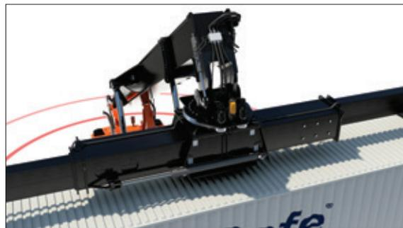
An antenna can be installed to the reachstackers spreaders or other attachments to create a moving detection zone.
