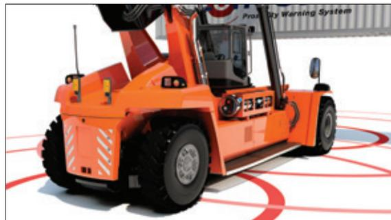
Two antennas have been installed at the back covering steer area of the reachstacker.
