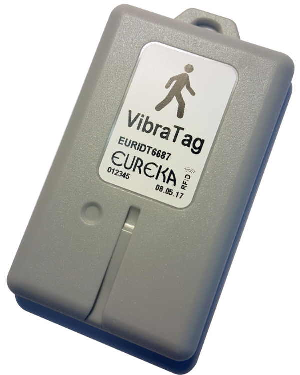
Back View - Clip can be fitted to the back of the tag as an optional extra (Part No. EURIDM6738).
