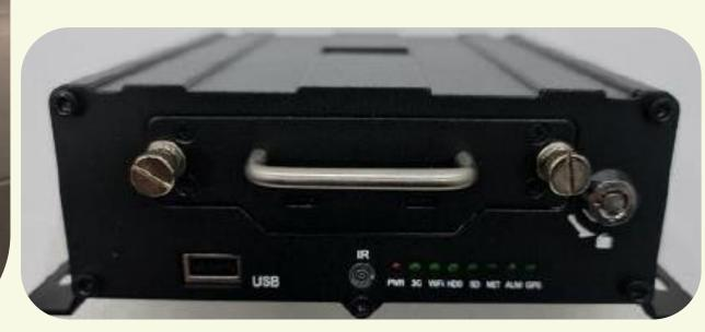
DBMS – System installed in vehicle to track and record driver behaviour data
